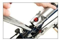
After installation, the status LED is not easily seen so it should be checked in a darker area. The status LED should light up for a moment every time the power adjuster is turned and every time a magnet passes the PAS and speed sensor.
