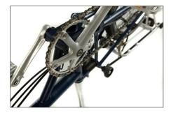
The magnet disc is simply slipped onto the shaft and positions itself when the crank is fastened. The magnet disc is now locked onto the square profiled shaft.
