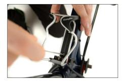
Fit the universal holder to the frame. Before doing so, the straps could be shortened provisionally to 14cm. When attaching the universal holder for the first time, make sure the straps are tensioned evenly. Whenever the bottle holder is fitted be sure not to forget the black abrasion protector. The washers serve no purpose.
