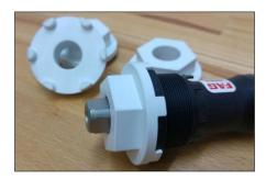
Please avoid the use of grips when removing the bottom bracket. We are able to offer the appropriate tools for every Brampton set. Please be aware that the bottom bearing has a left hand thread.
