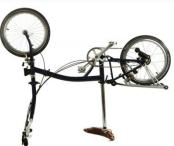
Note: If the bike is fitted with a mudguard, then this must be either removed or shortened appropriately. We would advise you to use the special tools required when dismantling the crank and bottom bracket. These tools can also be ordered from our shop.
