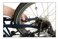
The exact positioning is done together with the spoke magnet. As shown in the picture, the sensor is mounted loosely on the frame with cable ties. These are then fastened properly when the positioning is finished. It is important to make sure that the connection wires do not rub on the wheel and that they are never under tension when the bike is folded.
