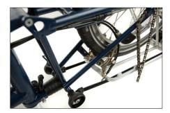
Remove the black stopper from the brake with a 10mm spanner. Then screw on the cap nut supplied together with the original washer.
