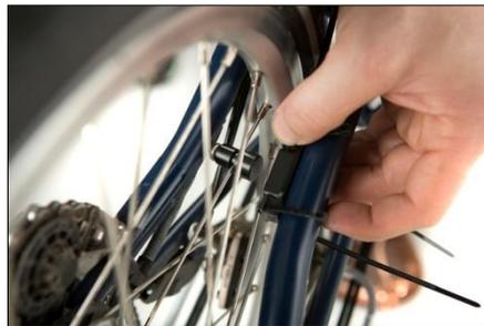
The spoke magnet should be fitted to the wheel opposite to the air valve. As shown in the picture, the spoke magnet must not be mounted on the same side of the wheel as the chain. The exact positioning is given when the sensor is attached to the frame. The gap between the spoke magnet and sensor should be approx. 1-2mm. The spoke magnet must not rub on the frame or sensor.
