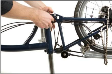
Be absolutely certain that wires cannot get caught up with the chain. When the bike is folded be sure that the wires cannot be pinched or torn out.
