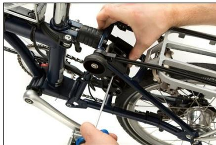
Fit the drive unit with the wires attached as there is little access to do it afterwards. Final adjustments will be done at a later stage.
