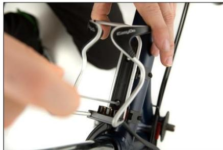
Fit the universal holder to the frame. Before doing so, the straps could be shortened provisionally to 14cm. When attaching the universal holder for the first time, make sure the straps are tensioned evenly. Whenever the bottle holder is fitted be sure not to forget the black abrasion protector. The washers serve no purpose.
