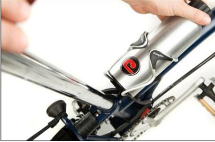
After installation, the status LED is not easily seen so it should be checked in a darker area. The status LED should light up for a moment every time the power adjuster is turned and every time a magnet passes the PAS and speed sensor.
