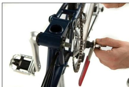
A crank puller is required to remove the cranks. Both cranks must be removed. If there is a cover present, this can be taken off with the aid of a small flat screwdriver.
