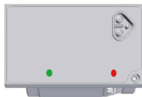
Speed sensor is recognised – green LED
