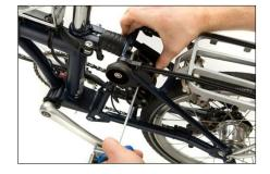
Fit the drive unit with the wires attached as there is little access to do it afterwards. Final adjustments will be done at a later stage.
