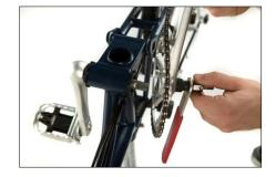
A crank puller is required to remove the cranks. Both cranks must be removed. If there is a cover present, this can be taken off with the aid of a small flat screwdriver.
