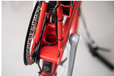
The battery cable should not shift
