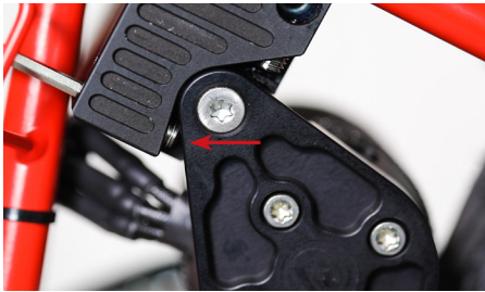
Screw just does not touch the swingarm
