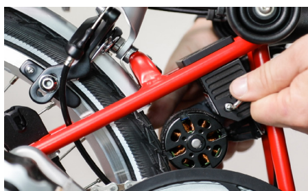
Loosen the freewheel setting screw
