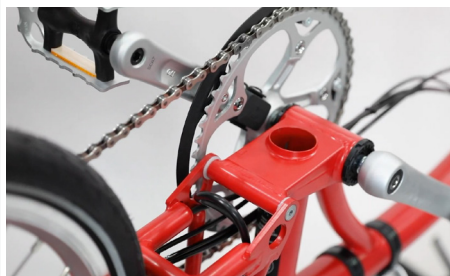
The battery cable is not pinched or kinked
