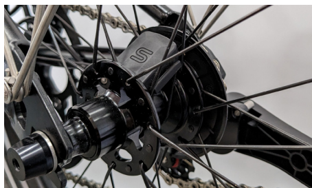
For P & T Line models speed sensor with slight angle
