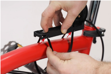
Wrap the steel straps around the bicycle frame
