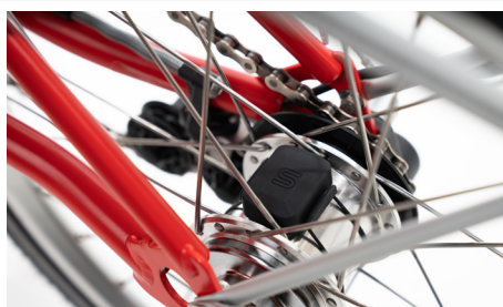
Speed sensor attached at rear wheel hub
