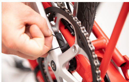
PAS sensor attached at the inside of the pedal crank
