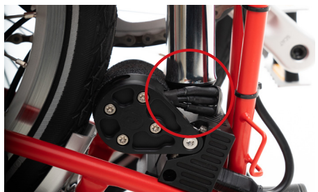
Rubber bumper press against the motor, cable must not be squeezed!
