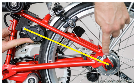
Imaginary line between the motor and the rear wheel
