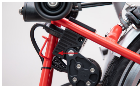
The electronics block rest gently against the frame
