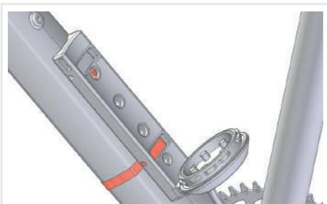
Attaching battery holder with screw & steel strap
