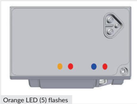
If the orange LED (5) flashes during the software update, it means the system cannot connect with the WiFi.
