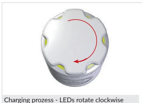
The clockwise rotation of the LEDs shows the charging speed and charging current. Towards the end of the charging process, the charging current and speed of rotation slow down until the charging process is finally completed and (if necessary) cell maintenance is initiated.
