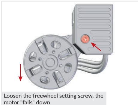
3. If the distance is less than 2-5 mm, loosen the freewheel setting screw (3) by one turn. You do not need to unscrew it completely.
