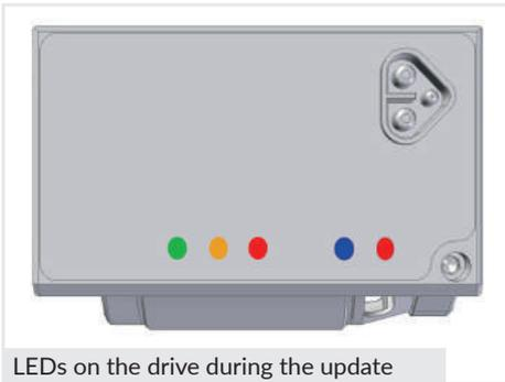
The following LEDs should be constantly lit on the drive while the update is being performed:
