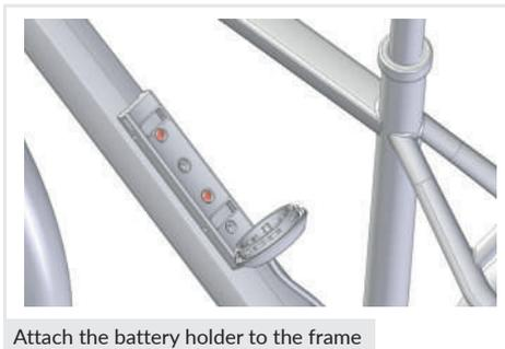
Attach the battery holder to the frame
