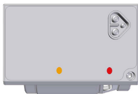
PAS is recognised – orange LED
